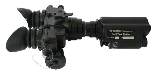
The OE-GNG Test Set is a hand-held, battery powered unit for field testing Night Vision Devices (NVD's). It is used by field personnel to determine the operational readiness of a NVD by checking its optical performance.
