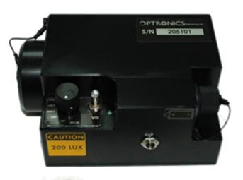
resolution adequacy, under low, high and 200Lux light levels. The OE-TSG-GNG Test Set uses a single 1951 US Air Force Resolution Test Target.
