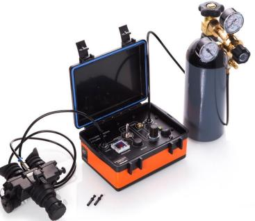
The system control unit performs air & nitrogen extraction, nitrogen fill-up, Leak testing (pressure maintenance) and High pressure purgation.
